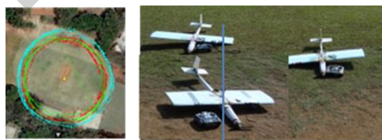
Figure 3: Three vehicles collaborating to fly in circle and maintain it during the flight
