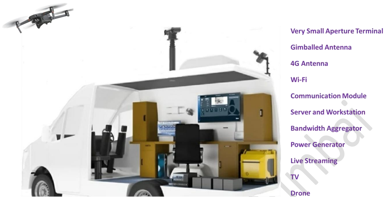
Figure 2: Proposed MCCC design, which is inspired by ground control station designed by DARC [1]
