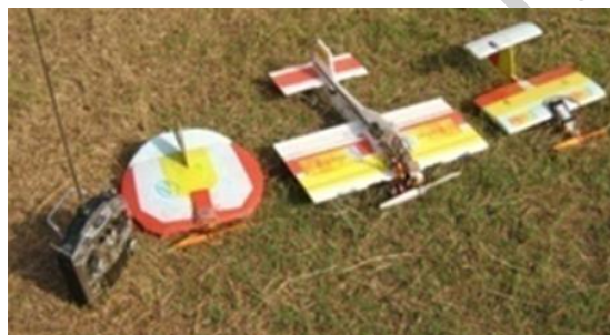
Figure 2: Autonomous electric powered UAS ~ 300 mm wing span
